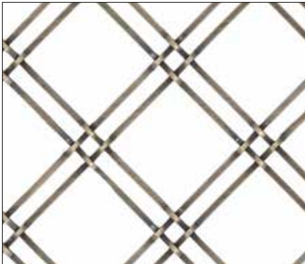
Press Crimped Square Wire .063" wire size, 1" & 1/4" mesh size
