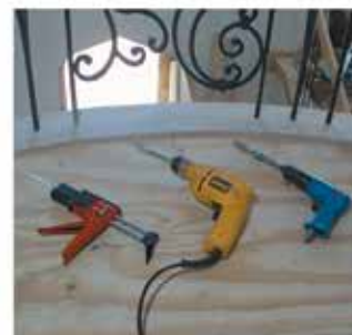
TOOLS USED: Standard Electric Drill, Air Hammer/Chisel, Epoxy Gun
